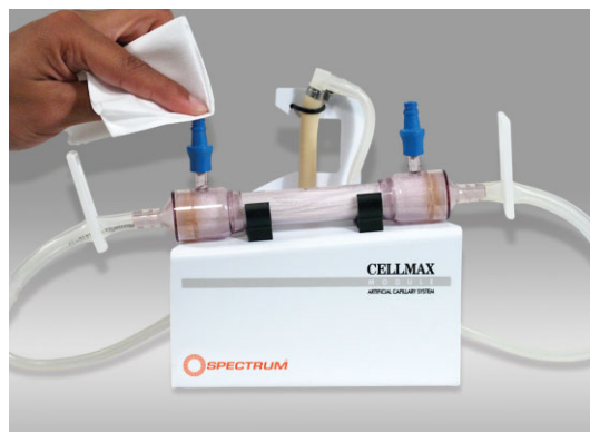
Figure 3: Disinfect side access ports
