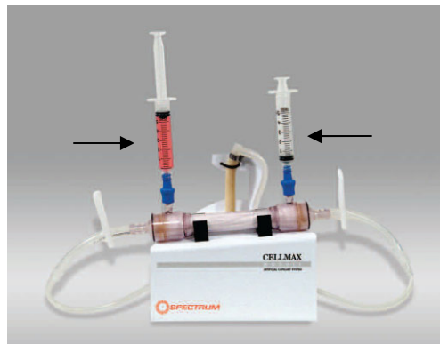
Figure 4: Attach syringe to side access port
