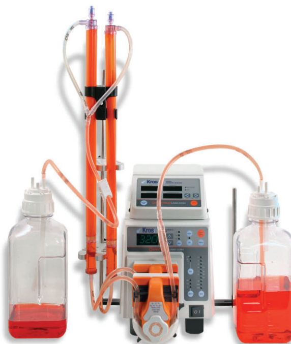
“Coupled” Tube-A-Lyzer® units set-up for parallel operation in single-pass mode.
